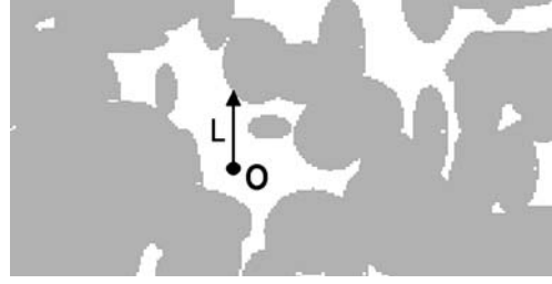
Figure 4. The random closed set \Xi is shown in grey. If o does not belong to \Xi consider the vertical line L from o to the first contact with \Xi . The length of this line segment is a random variable with linear contact distribution function.
